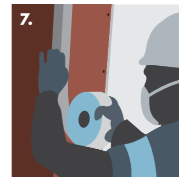
7. Taping and jointing encasement corners
