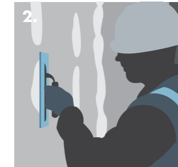
2. Applying Knauf Plasterboard Adhesive dabs at the required centres.
