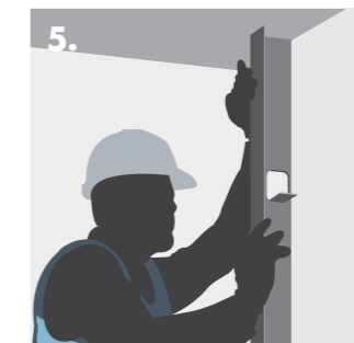
5. Knauf 'J' Channels are used vertically at corners and abutments.
