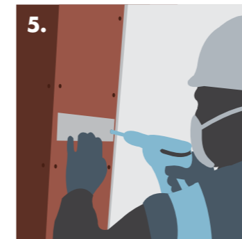
5. Fixing Knauf Flat Fixing Plate between layers.
