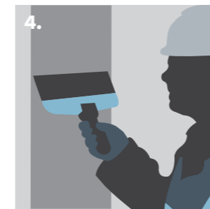
4. Applying the first coat of Knauf Joint Cement Easy Sand.
