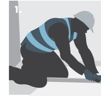
1. Scoring Knauf Aquapanel Exterior with a knife.
