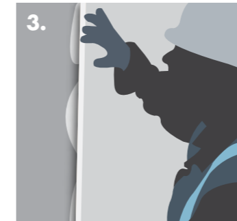
3. Offering up Knauf Plasterboard and pressing into place.
