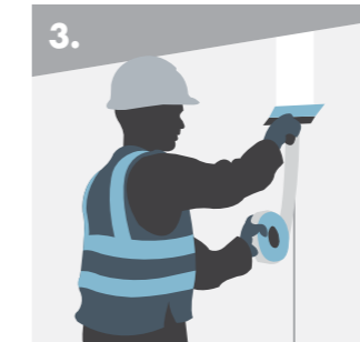
3. Embedding Knauf Aquapanel Exterior Joint Tape.
