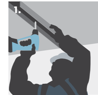
1. Fixing Knauf 'J' Channel to the soffit.
