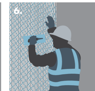
6. Applying reinforcing mesh.
