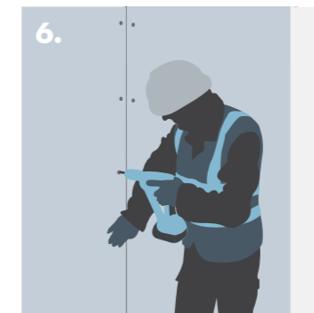
6. Fixing Knauf Soundshield Plus to the frame.
