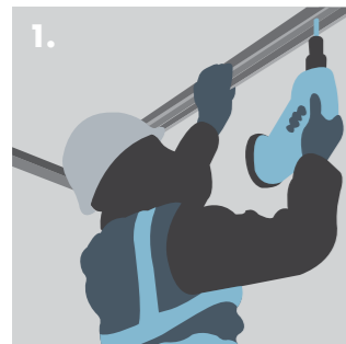
1. Fixing Knauf 'U' Channel – Perimeter Support to the soffit.
