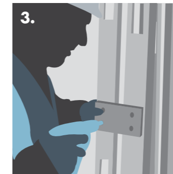
3. Bracing Knauf 'C' Studs with Knauf Fixing Channel at maximum 1500mm vertical centres (if required).
