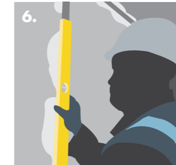
6. Ensuring Knauf Metal Furring Channels are fixed plumb.
